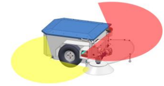
CAD robot model with lidar field of view
