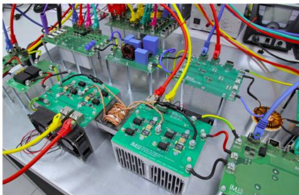
Fig. 10: Rapid prototyping environment with GaN full bridge modules and transformer of DAB in the front
