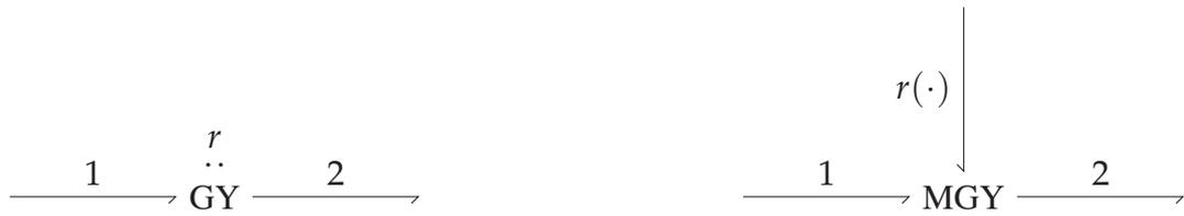
Figure 4.7.: Representation of a two-port gyrator
