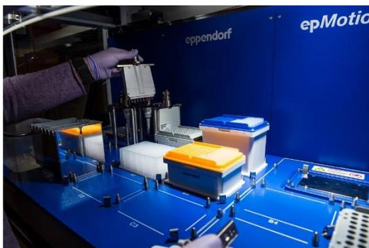
epMotion – Automated Liquid Handling system by Pacific Northwest National Laboratory (PNNL), CC BY-NC-SA 2.0
