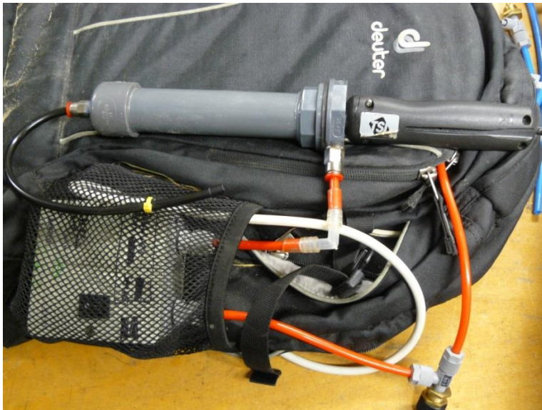
Figure 9: CO 2 probe inserted into sampling chamber.
