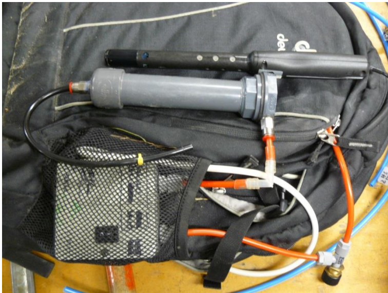
Figure 8: CO 2 probe and sampling chamber.
