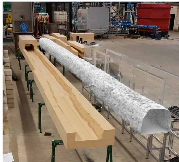
Scale model production of an unlined rock blasted tunnel (white structure shows the digital elevation model of the tunnel). (Photo: R. Eikenberg)
