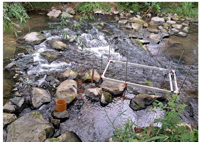
Velocity measurements in the field over an unstructured block ramp (Photo: R. Eikenberg)
