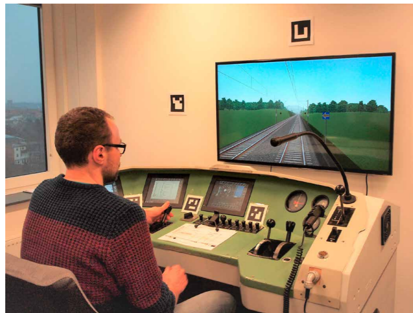
This Side: Train driving simulator in the Virtual Railway Operations Laboratory (Bildautor: Pachl)
