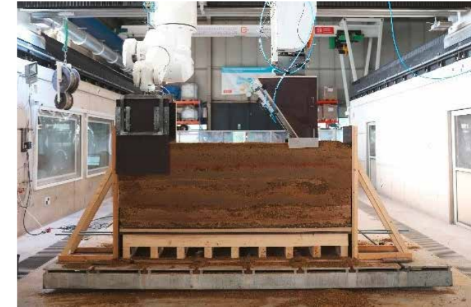
Additive Manufacturing with earthen materials left: Sprayed Earth Additive Manufacturing; right: Robotic Rammed Earth
