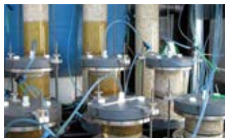
Filtration experiments to remove mercury from contaminated groundwater by means of amalgamation on brass.
