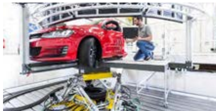
Dynamic Vehicle Road Simulator for Testing Intelligent Vehicle Systems © NFF/Bierwagen
