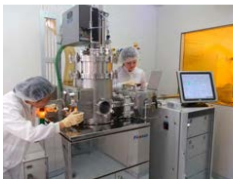
Members of the Institute of Semiconductor Technology are coating nanostructures using an atomic layer deposition (ALD) system.
