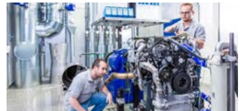
One of 16 Engine Test Benches in Use at the NFF © NFF/Bierwagen
