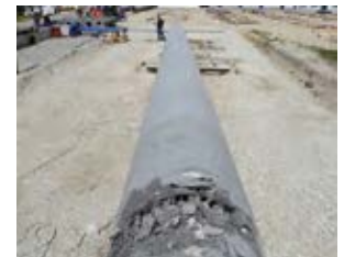
Slender spun concrete pole after testing
